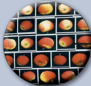
Our module for external quality (iQS - intelligent Quality Sorter) sorts the fruits automatically by taking about 70 pictures of each fruit. This is done using special infrared and colour cameras. The advanced software analyses the pictures and classifies them according to the programming of the operator.
