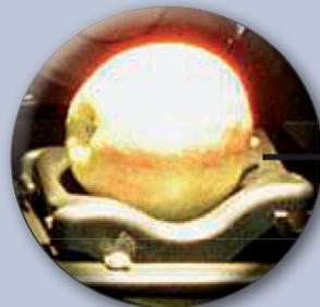
iFA assesses the internal quality of the fruit. A halogen light source is used for a measurement by means of iFA. The fruit is 'X-rayed' by the beam of light. On the basis of a spectrum analysis, a forecast is made with respect to brix value, internal brownness and core rot. This analysis gives an assessment of the entire piece of fruit instead of just a small part of it.
