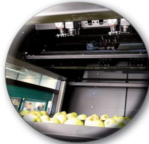
GeoSortIII is a high-end sorting machine which sorts no less than 8 fruits per second. It also handles your fruit with great care. The GeoSortIII is therefore particularly suitable for easily bruised fruit, e.g. delicate apples such as Golden Delicious or peaches.
